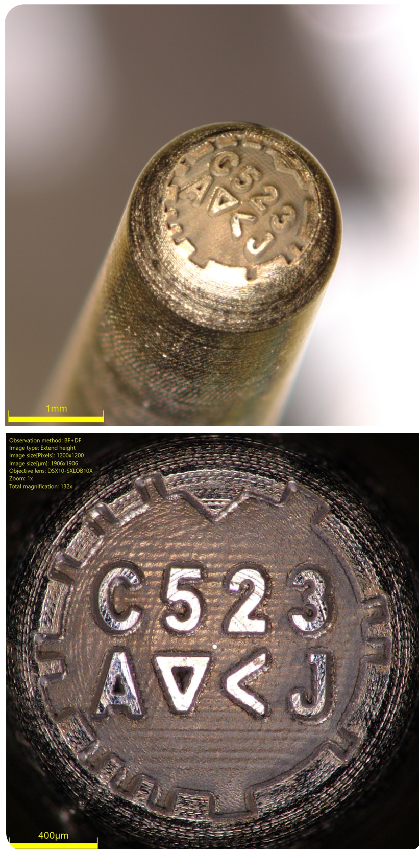
Figure 3: A firing pin equipped with microstamping technology.
